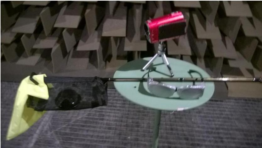
*Figure 1. The direction-pointing test equipments: Bluetooth loudspeaker in a pouch and bright-coloured flag on tip of a short fishing rod, video camera and blinding eye glasses.*
